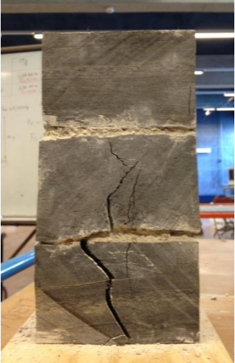
Figure 8: Sample of a schist triplet after failure.
