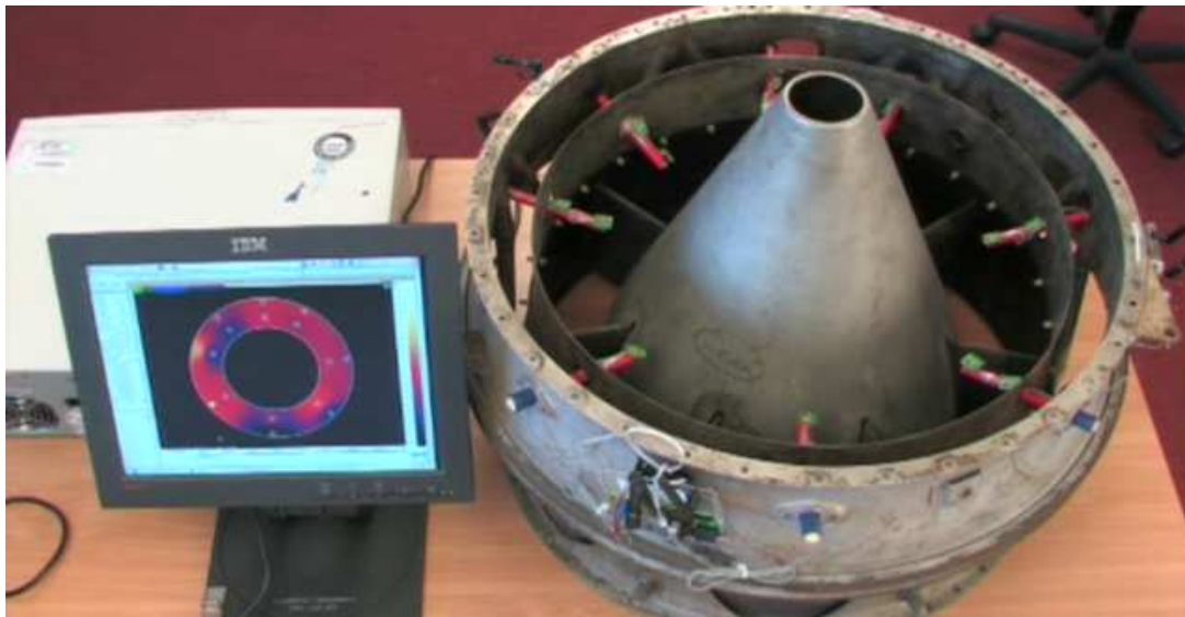
Figure 16: Base station and instrumented gas turbine engine
