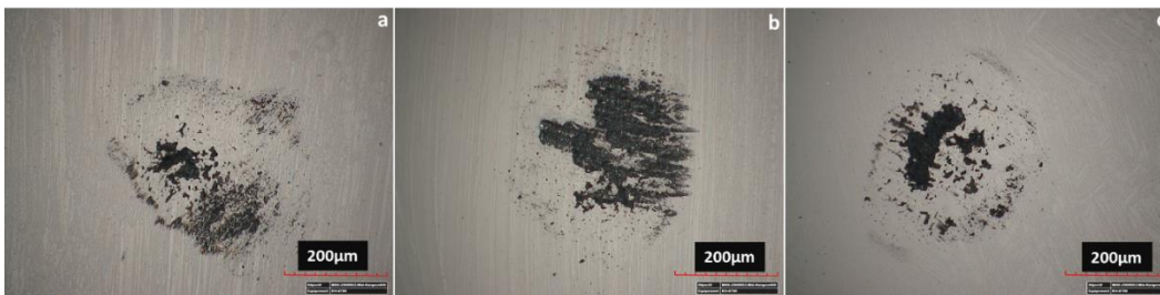
Fig. 5 - Optical microscope surface of testing alumina balls after the dry sliding friction test. (a) electroless NiB without ultrasound, (b) electroless NiB with 20 kHz frequency and 0.058 \text{ W/cm}^3 energy density ultrasound, (c) electroless NiB with 35 kHz frequency and 0.065 \text{ W/cm}^3 energy density ultrasound.
