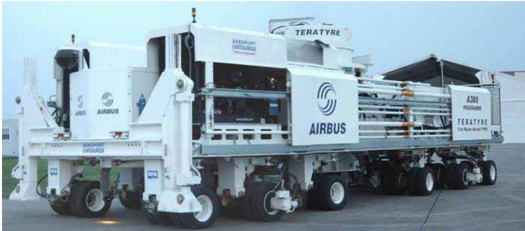
Figure 3: Airbus TERATYRE (Test Rig for Aircraft TYRE) Machine [10]
