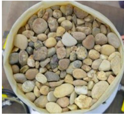
Figure 8: Granular backfill used in the experiments by Colas [12].
