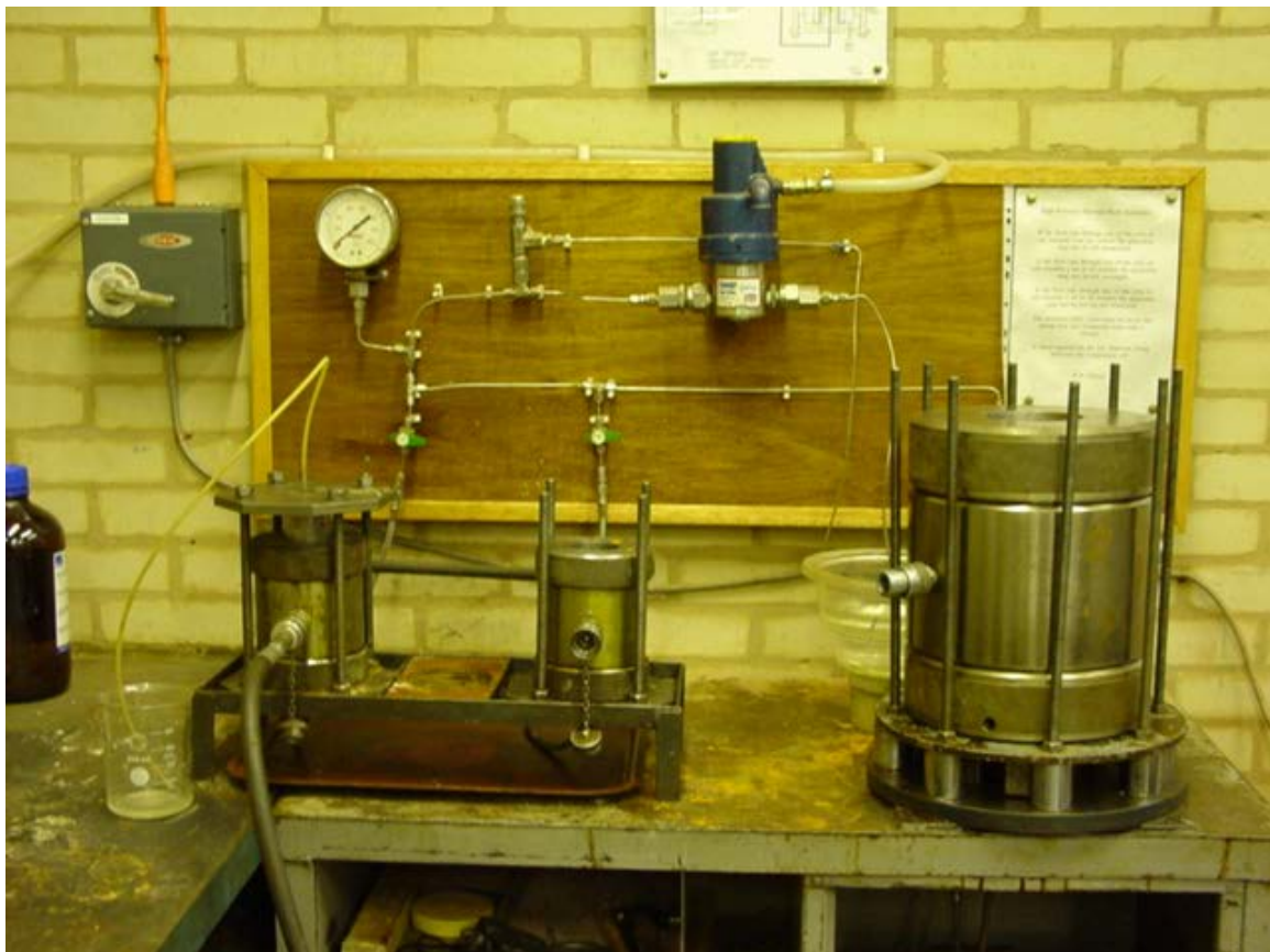
Fig. 2: High-pressure apparatus at Coventry, showing two small cells (for 54 mm diameter samples) and one big cell (for 100 mm diameter samples) together with liquid pump and pressure gauge.
