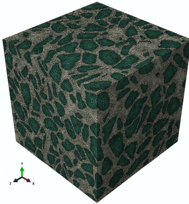
Fig. 15 The finite element mesh for the 37mm concrete cube
