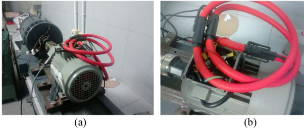
Fig. 1. Experimental test bench: a) motor-load bench and b) the current clamps configuration.
