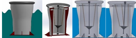
Figure 3: A fully enclosed multi axis combined surge and pitch WEC.
