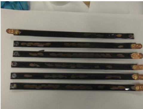
Fig. 15. Aged samples at 275°C after 400hrs.
