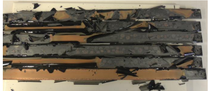
Fig. 3. Catastrophic insulation failure of samples at 260°C after 1600 hours.
