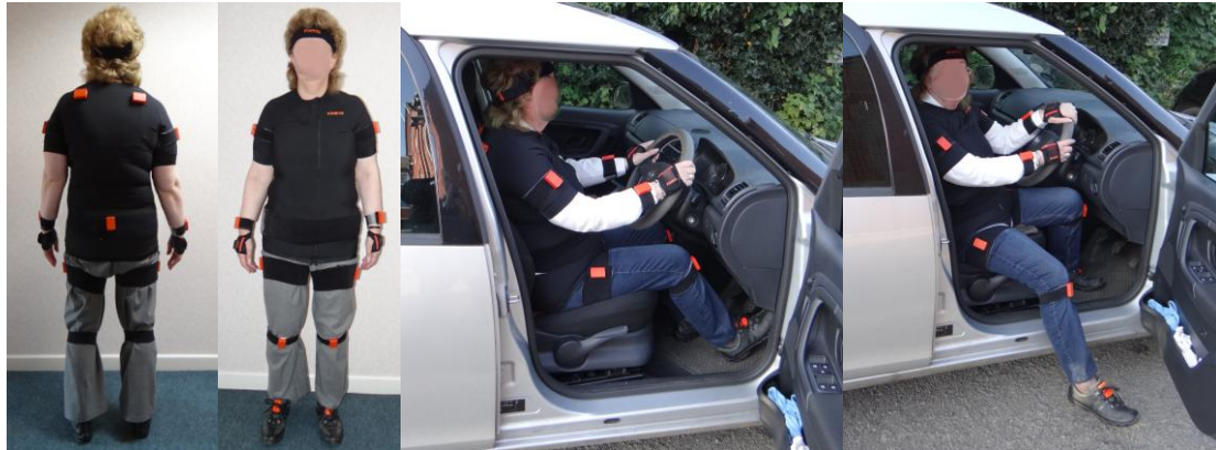
Figure 1: Magneto-inertial motion capture system attached to a subject – the sensors are the small “matchboxes” attached to the subject
