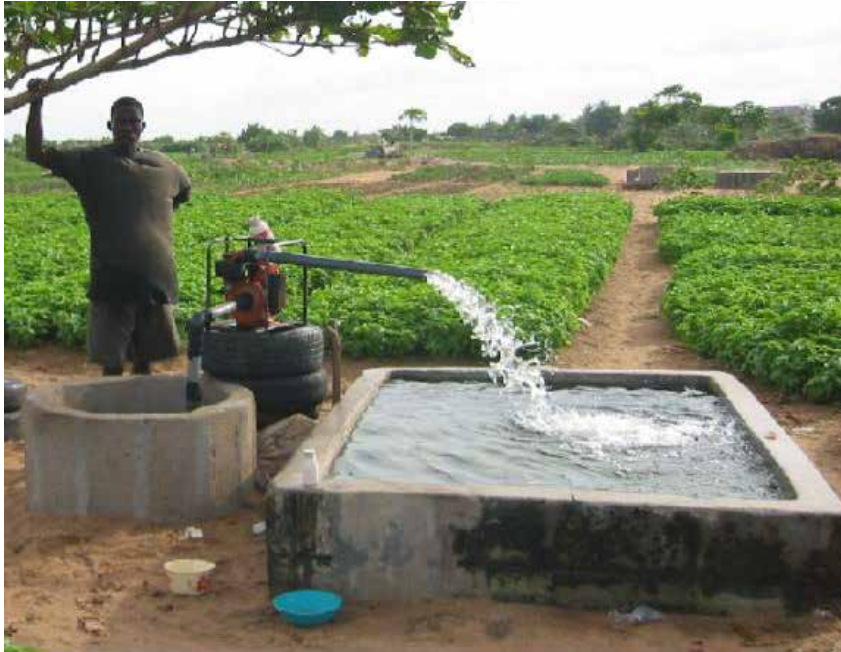
FIGURE 7.5. Watering can irrigation with well, pump and storage reservoirs in Togo. Other reservoirs are visible in the background (photo: IWMI).
