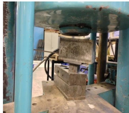
Figure 2 50mm cube compaction at 52kN
