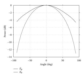
FIGURE 14: Radiation pattern of circular waveguide at  $r=0.5\lambda$  (1.6 cm).
