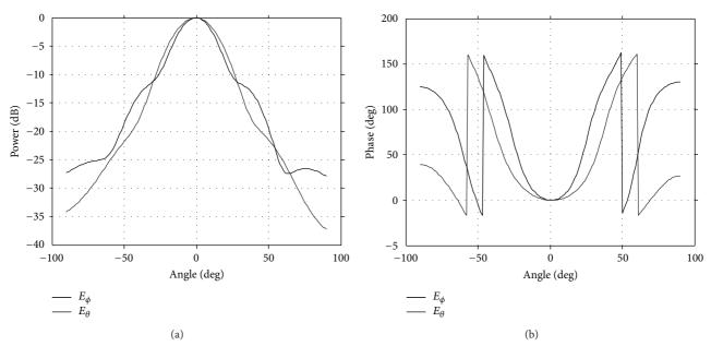
FIGURE 24: (a) Radiation pattern of conical horn at  $r = 10\lambda$  (32 cm). (b) Phase pattern of conical horn at  $r = 10\lambda$  (32 cm).
