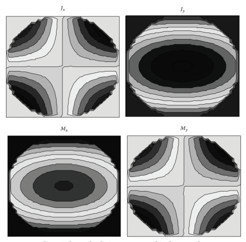
FIGURE 3: Current distribution over aperture of circular waveguide.
