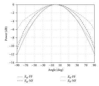
FIGURE 8: Comparison of far field (FF) and near field (NF) pattern of circular waveguide at  $r=D^2/\lambda$ .
