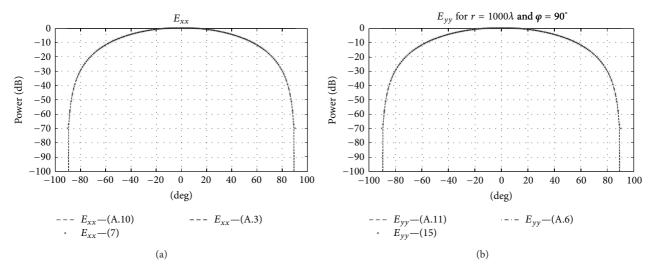
FIGURE 25: (a) Comparison of copolar ( $E_{xx}$ ) component of x-directed electric point dipole in  $\varphi = 0^\circ$  plane;  $\lambda = 3.2$  cm. (b) Comparison of copolar ( $E_{yy}$ ) component of y-directed electric point dipole in  $\varphi = 90^\circ$  plane;  $\lambda = 3.2$  cm.
