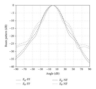
FIGURE 18: Comparison of near field and far field radiation patterns of conical horn (radius =  $4.1 \, \text{cm}$ ; semiflare angle  $\alpha_0 = 21.09^\circ$ ).
