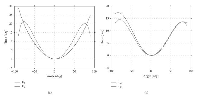
FIGURE 10: (a) Phase radiation pattern of circular waveguide at  $r = D^2/\lambda$ . (b) Phase radiation pattern of circular waveguide at  $r = 2D^2/\lambda$ .
