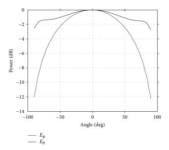
FIGURE 7: Radiation pattern of circular waveguide at a distance of  $D^2/\lambda$ .
