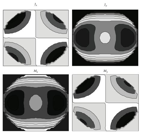
FIGURE 4: Current distribution over aperture of conical horn.
