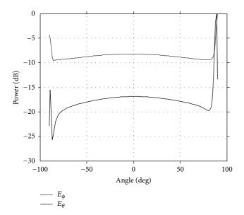
FIGURE 11: Near field radiation pattern of circular waveguide at  $r=0.2\lambda$  (0.64 cm).
