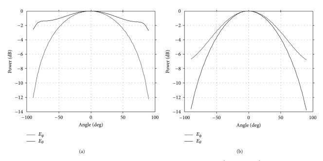
FIGURE 9: Amplitude radiation patterns of circular waveguide. (a)  $r = D^2/\lambda$ ; (b)  $r = 2D^2/\lambda$ .
