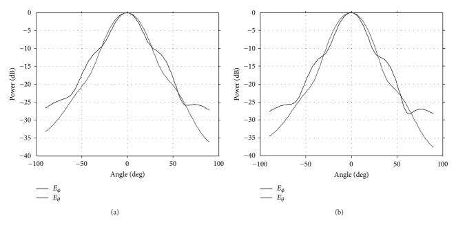
FIGURE 19: Comparison of amplitude radiation pattern of conical horn: (a)  $r = D^2/\lambda$ , (b)  $r = 2D^2/\lambda$ .
