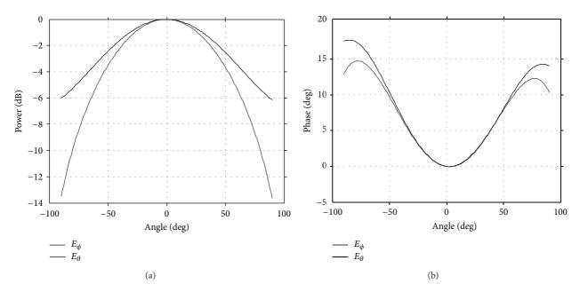
FIGURE 15: (a) Radiation pattern of circular waveguide at a distance  $r = 0.75\lambda$ . (b) Phase pattern of circular waveguide at a distance  $r = 0.75\lambda$ .
