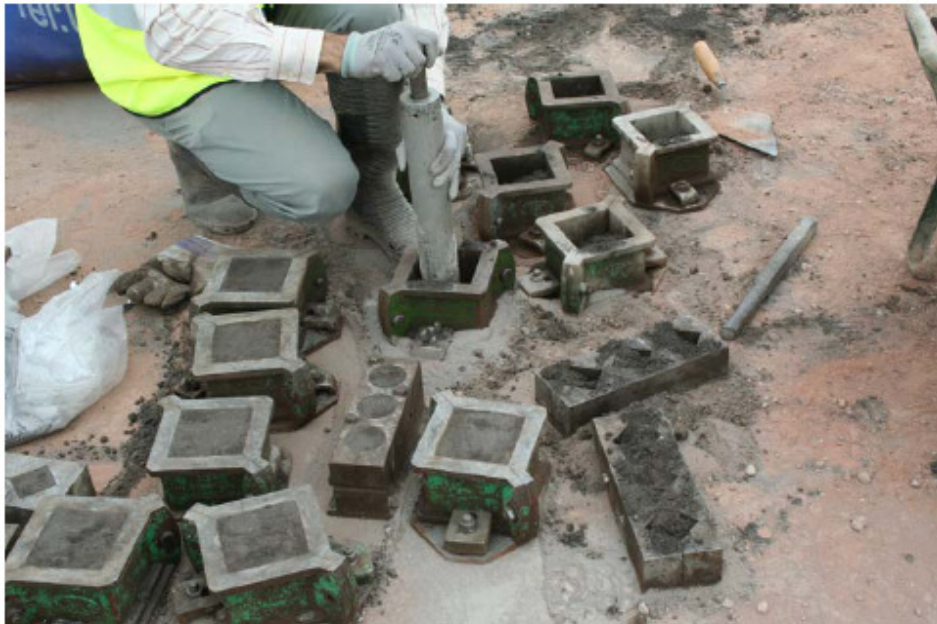
Figure 119. Sampling the semi-dry paste using 100 and 50 mm cubes.
