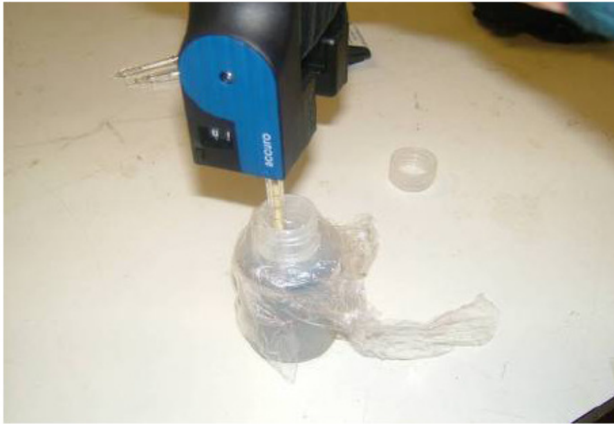
Figure 70. Testing the paste samples using the H 2 S detection tube
