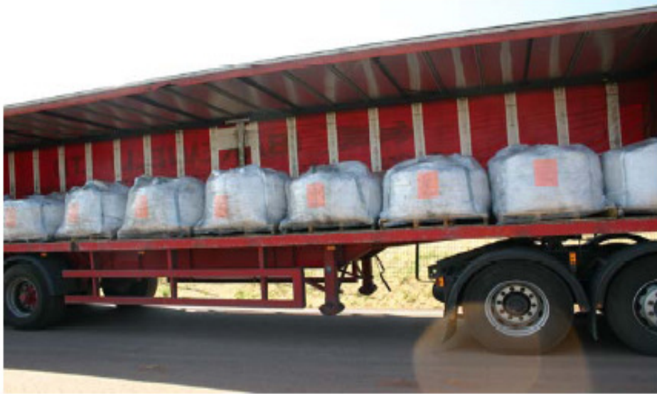
Figure 85. Blended powder delivered to the King's Mill Hospital site in 1000-kg sling bags.
