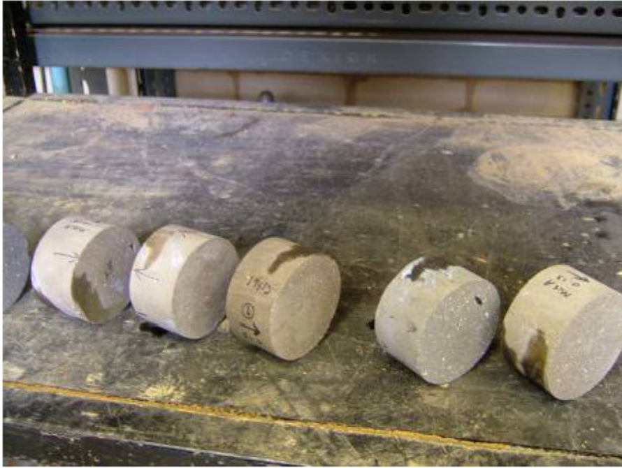
Figure 73. Paste specimens prepared for high pressure through-flow test.
