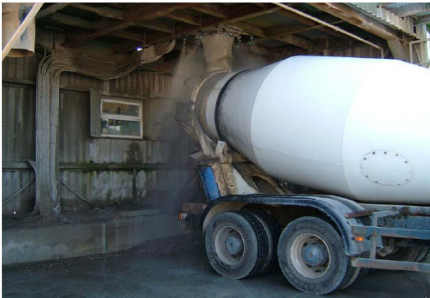
Figure 89. Loading aggregates and water into the truck mixer.
