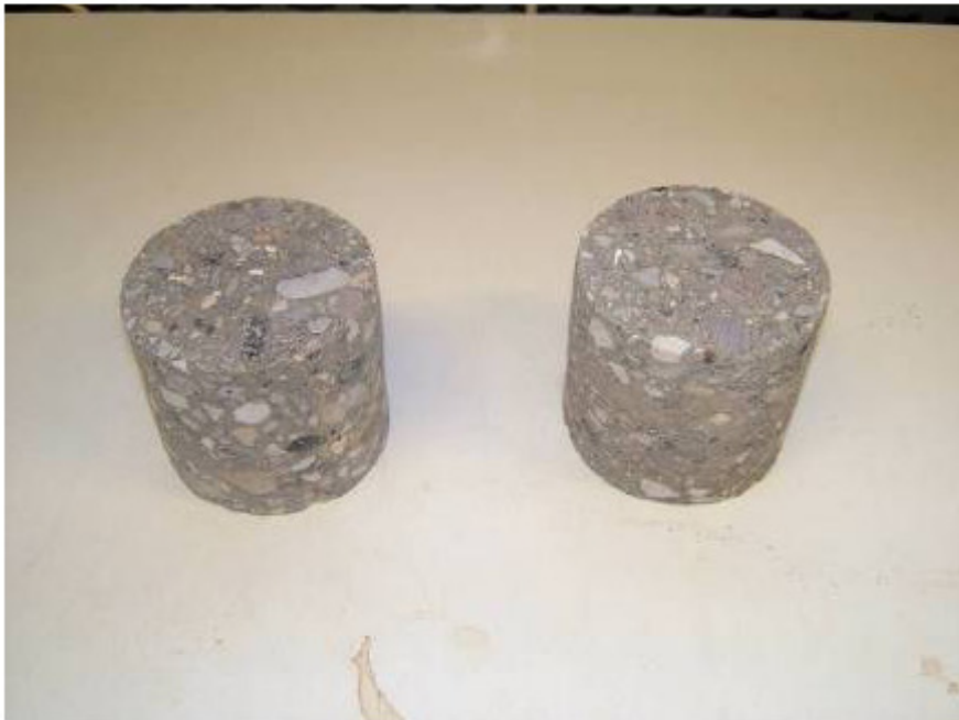
Figure 129. RCC core samples taken from different locations of the trial car park at the Lowdham Grange site.
