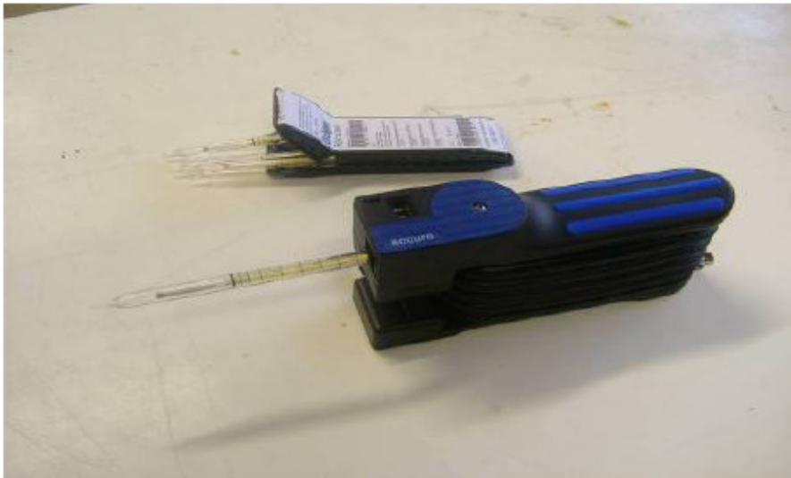
Figure 69. Drager Accuro pump kit and H 2 S detection tube.
