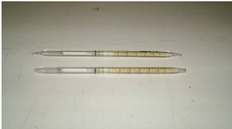
Figure 71. Comparison between new and used H 2 S detection tube for mix containing 50% paper.
