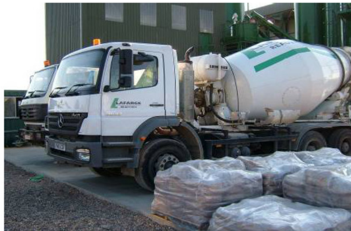
Figure 84. Blended powder delivered to the ready-mix plant in 20-kg bags.
