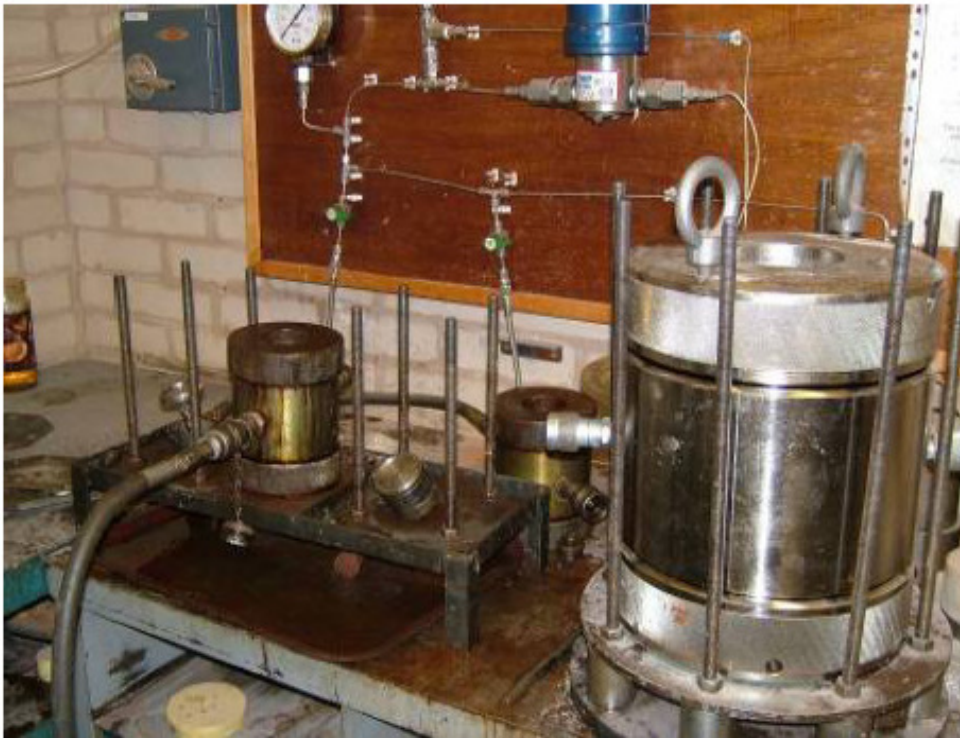
Figure 72. Hoek cells used for high pressure through-flow test.
