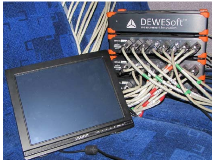
Figure 1. Sirius data acquisition system used for measuring the acceleration at locations on the bus where the kinetic energy recovery system may be installed.
