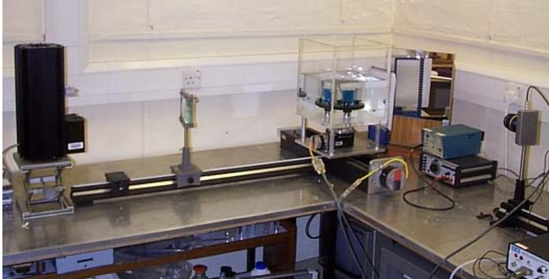
Fig. 3. Photograph of the acquisition portion of the CCD optical tomography scanner
