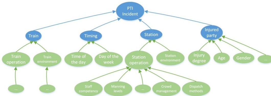
Figure 4. A section of the Platform-Train Interface safety incident model as outlined by experts during the knowledge elicitation exercise.
