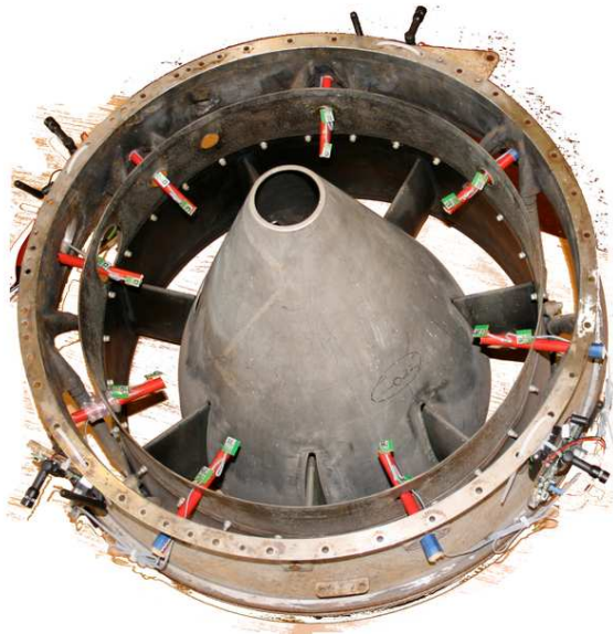
Figure 2.18: Annulus with I 2 C sensors and Gumstix attached
