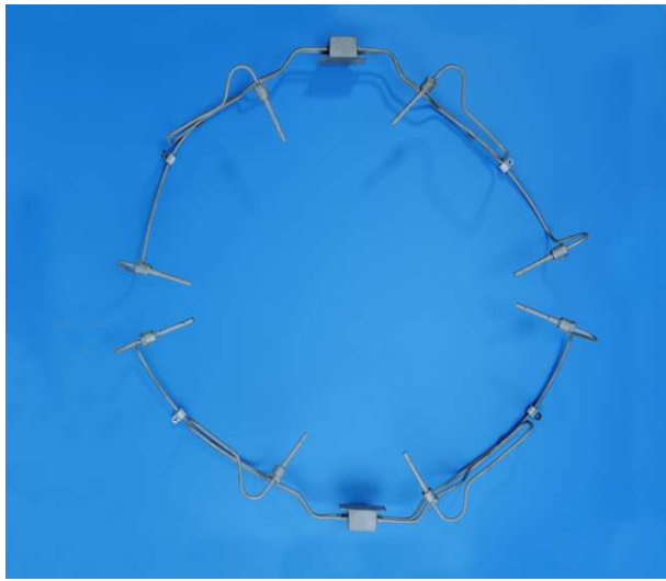
Figure 2.17: Annulus thermocouple harness (picture supplied by Vibro-Meter UK)
