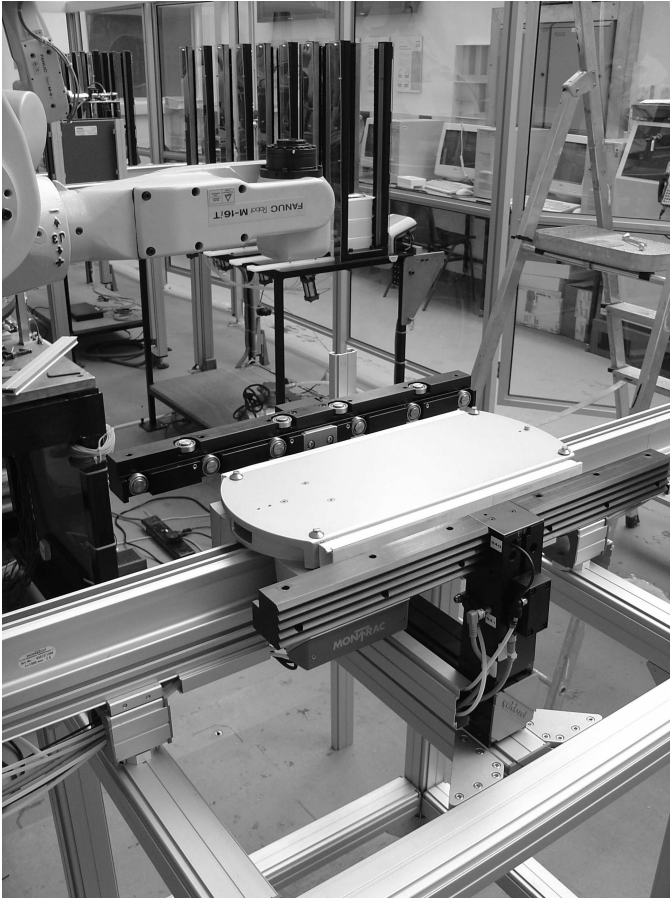
Fig. 10. Photograph of docking station, also showing a shuttle (without a top).
