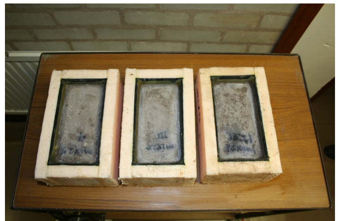
Fig. 3. Specimens for freeze/thaw test
