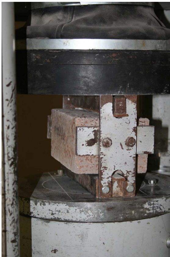
Fig. 2. Steel frame of split tensile strength test
