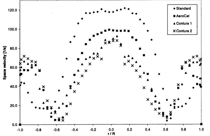
Figure 9. Flow distribution at  $Re \approx 85000$
