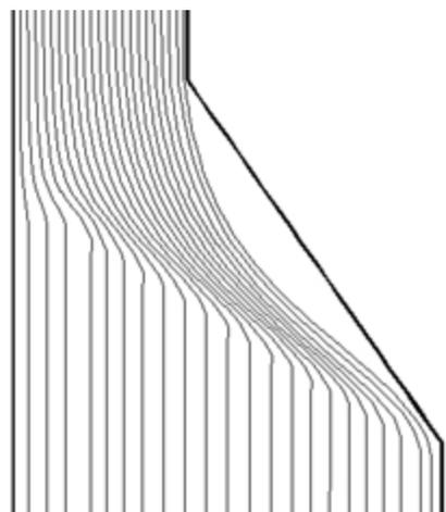
Figure 19. Particle tracks for the Contura 1 geometry
