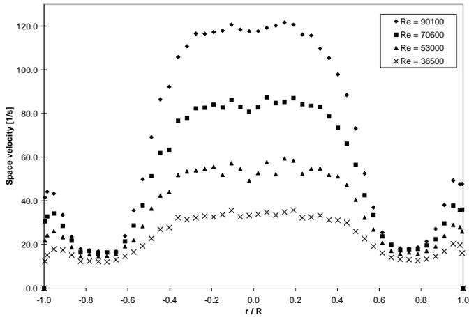
Figure 5. Flow distribution for the Standard substrate
