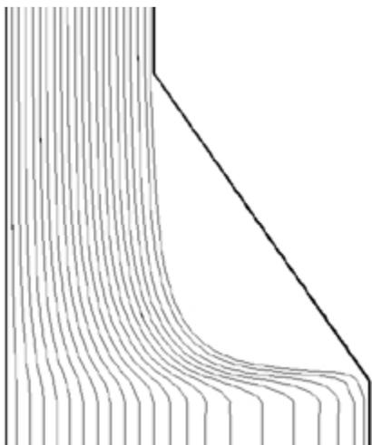
Figure 18. Particle tracks for the Standard substrate geometry
