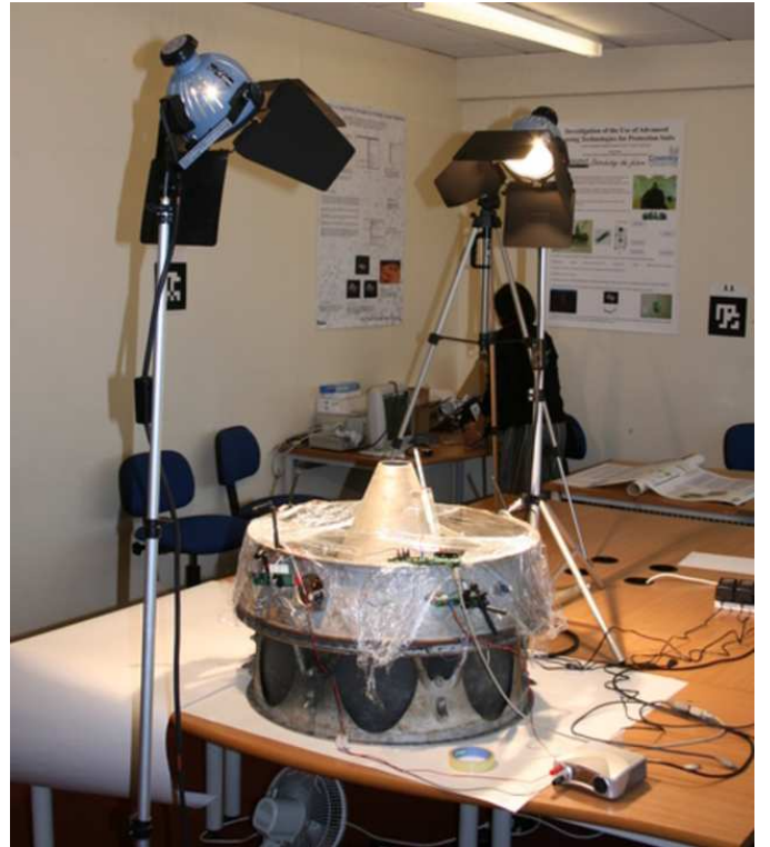
Figure 9. Experimental configuration including lights to heat pipe section and polyurethane film used to reduce airflow.
