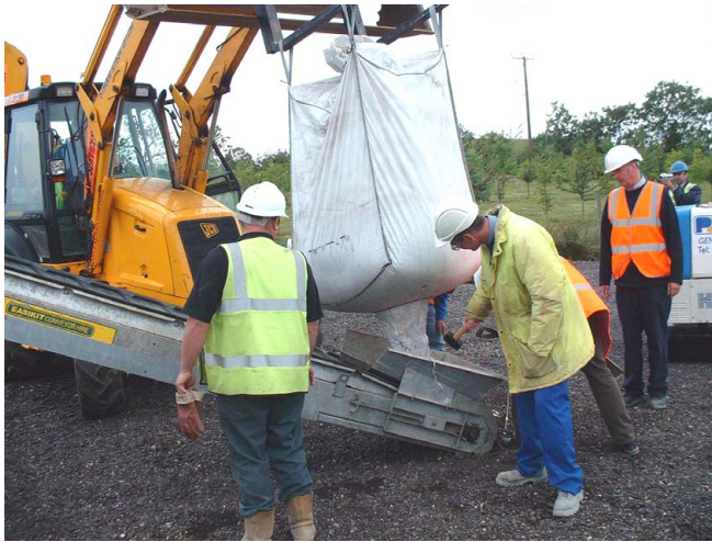
Fig. (18). BOS Slag discharge to conveyor.
