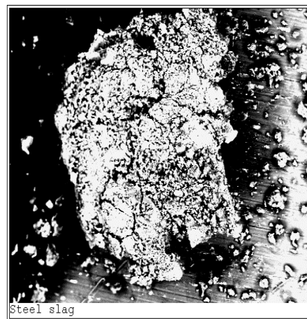
Fig. (3). BOS slag grain. Left: Secondary electron image showing surface morphology, right, backscattered electron image showing fracture porosity within the grain. As the efficiency of electron backscattering is a function of the average atomic number of the target, the technique reveals the internal fractures within the slag grain.
