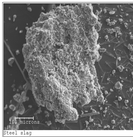
Fig. (3). BOS slag grain. Left: Secondary electron image showing surface morphology, right, backscattered electron image showing fracture porosity within the grain. As the efficiency of electron backscattering is a function of the average atomic number of the target, the technique reveals the internal fractures within the slag grain.
