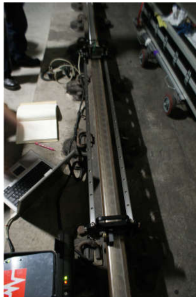
Figure 1 Photograph of ODS wheel and rail roughness measuring system.
