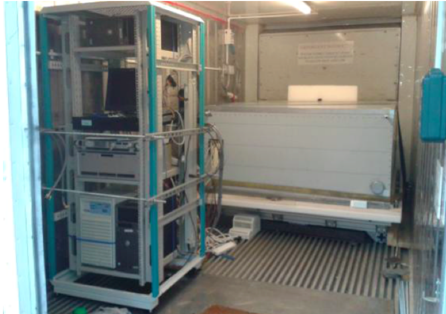
Figure 1. The detector inside the refrigerated 20 ft. ISO shipping container, showing the size and footprint of the detector itself. The rack in the foreground contains services and DAQ systems for readout.
