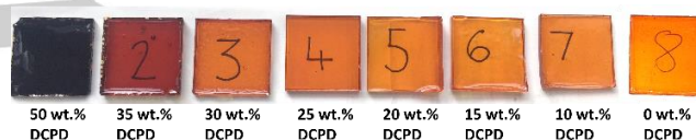
Figure 8: Photographs of ~5 mm thick blocks of polymers made from 50 wt.% sulfur and 50 wt.% crosslinker, where the crosslinker was composed of copolymers of DCPD and terpinolene, going from all DCPD (left) to all terpinolene (right). Numbers written in pen under the samples can be read clearly for most samples.
