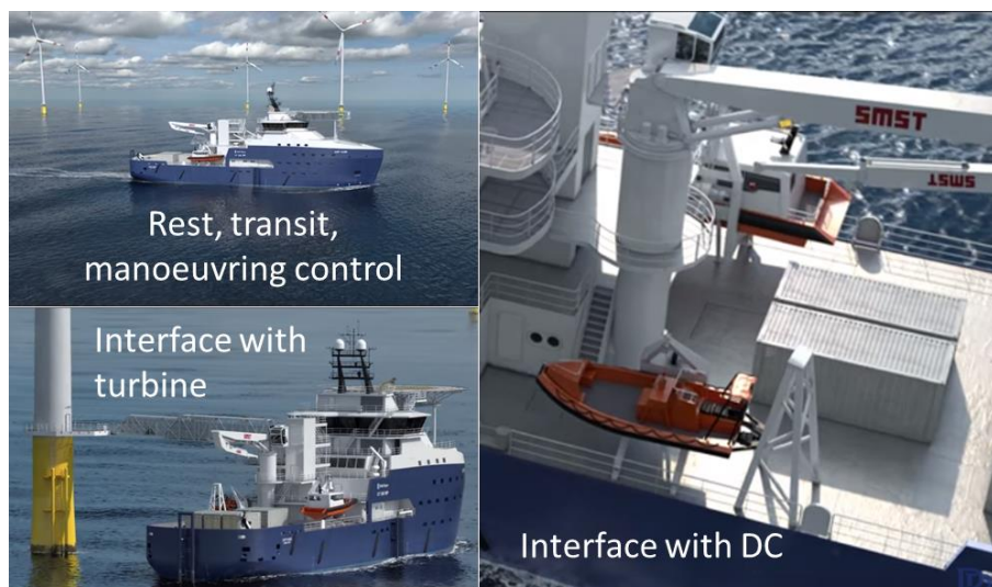
Figure 1: Operation modes when DP system is used (courtesy of Kongsberg Maritime / fmr Rolls-Royce Marine)
