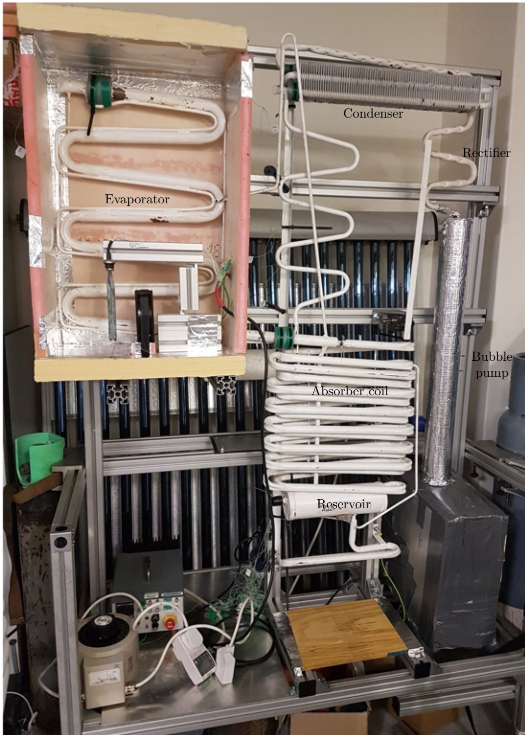
Figure 2. Photograph of the laboratory DAR system used in the experiments.
