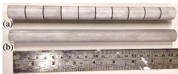
Figure 1. Model piles used in centrifuge test (a) low stiffness pile and (b) continuous high stiffness pile.
