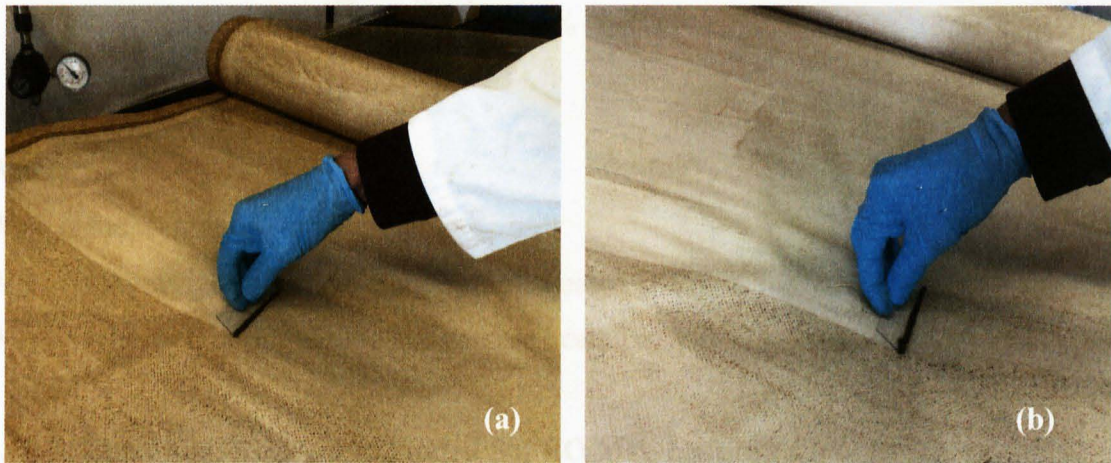
Figure 3.12: Photographs of scraping of fouling material from the surfaces of Fluid Systems (a) and Toray (b) SWRO membranes
