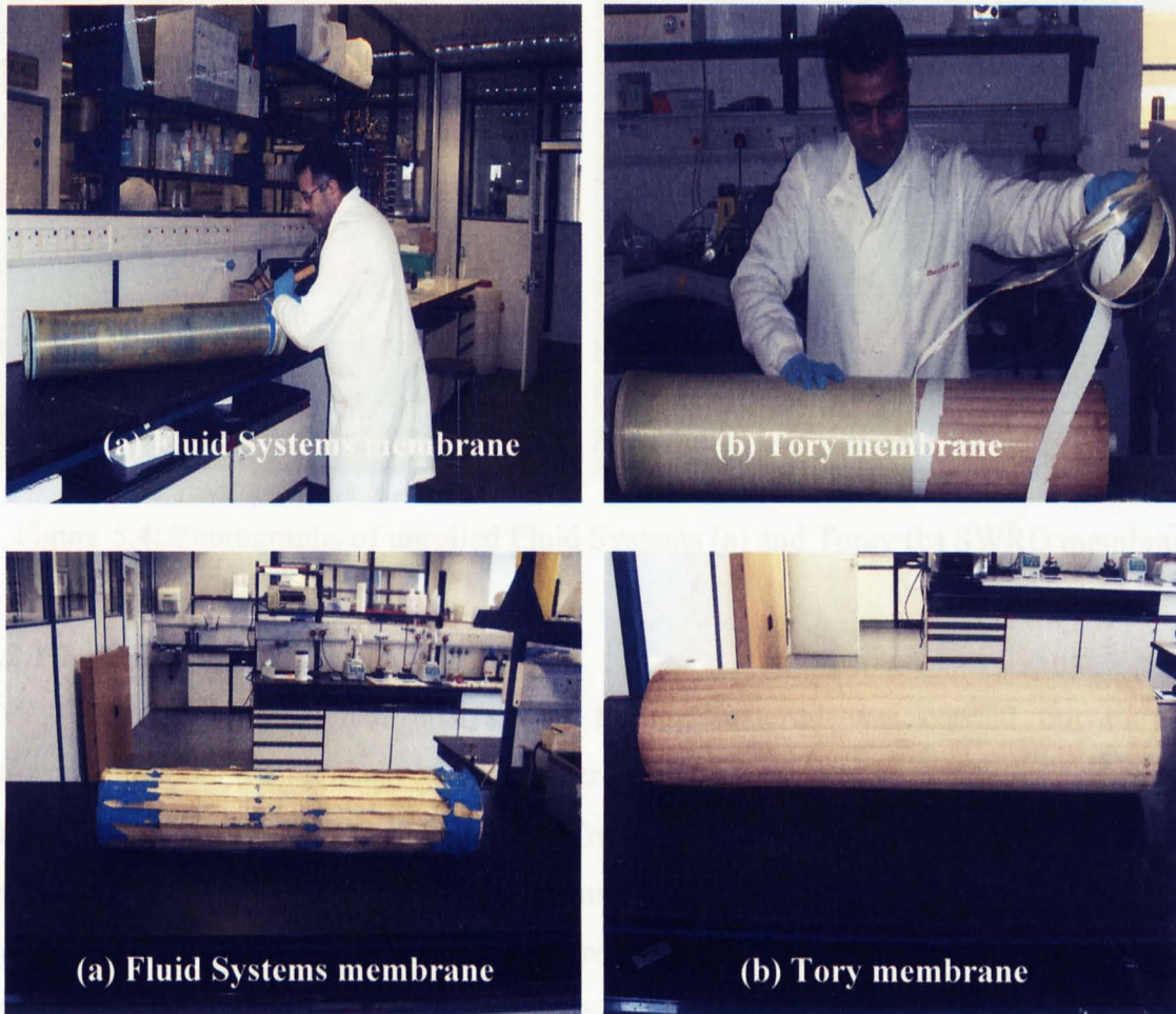
Figure 5.3; Photographs of the Fluid Systems (a) and Toray (b) SWRO membrane before and after removing the end caps and plastic casing.
