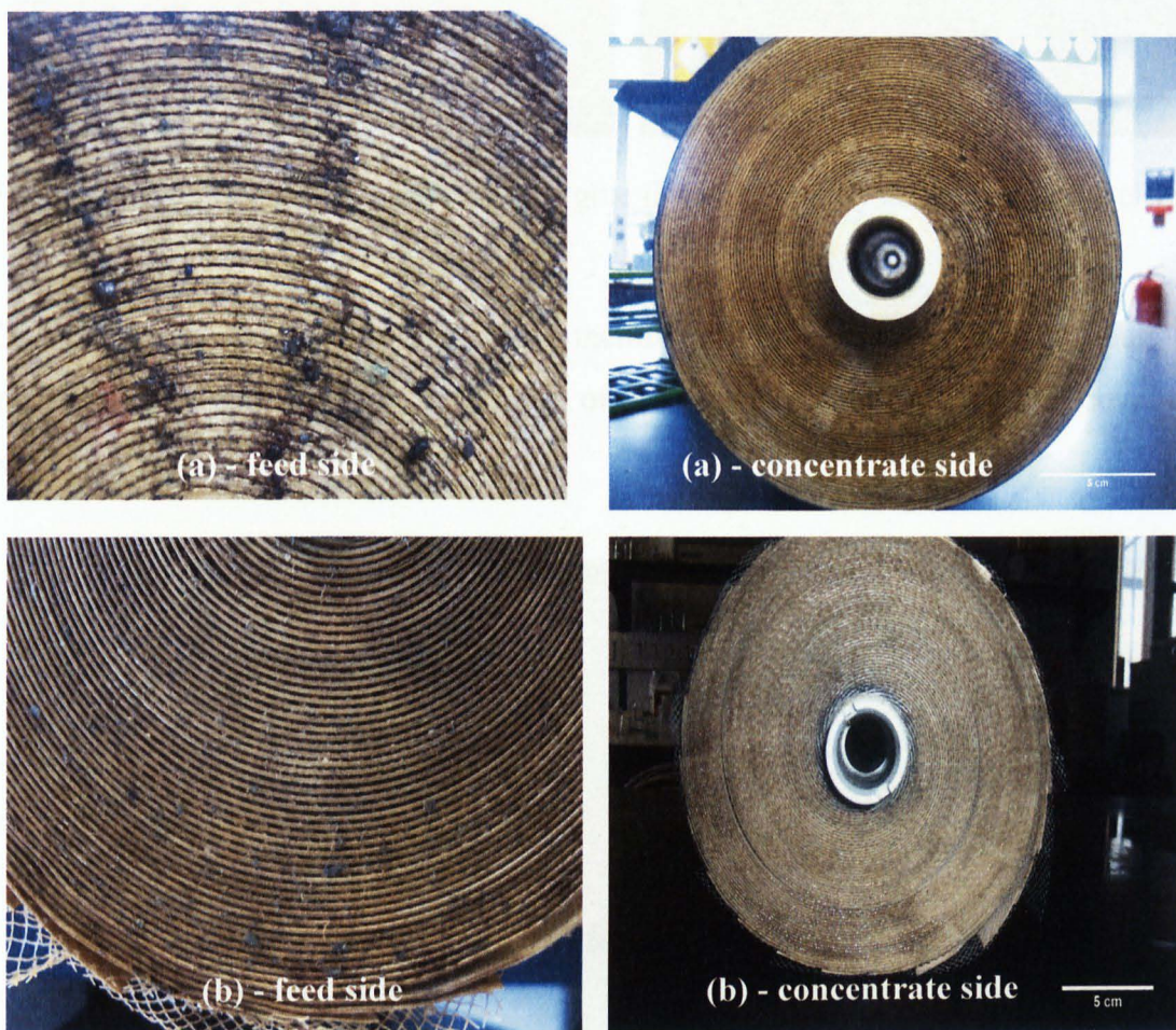
Figure 5.5: Photos of feed and concentrate sides of Fluid Systems (a) and Toray (b) membrane elements.
