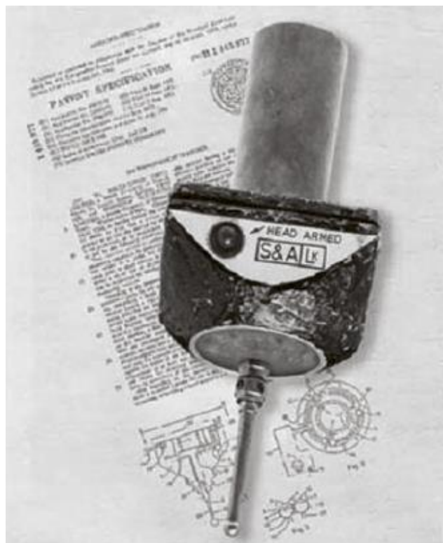
Figure 31: The original three dimensional touch trigger probe invented by Sir David McMurtry in 1972 [282].
