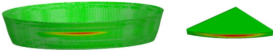
Figure 51: Wear measurement narrowed down from full liner to wear sector in order to limit the errors induced.
