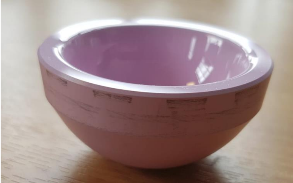
Figure 53: Image displaying wear at the clamping area on the exterior part of the liner.
