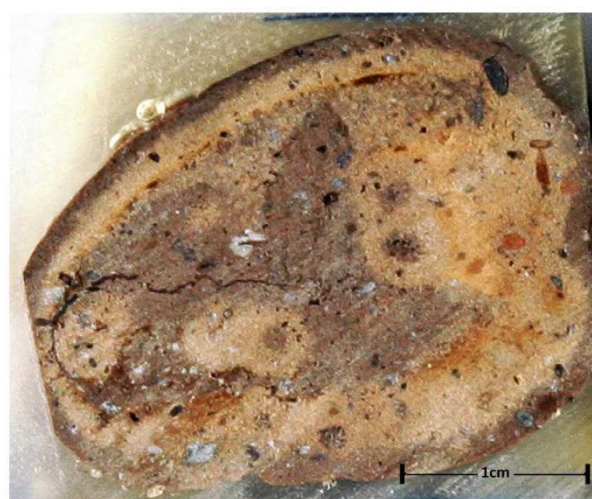
Figure 2. Several inclusions can be seen on the surface of a cross section of sample PHL-60.
