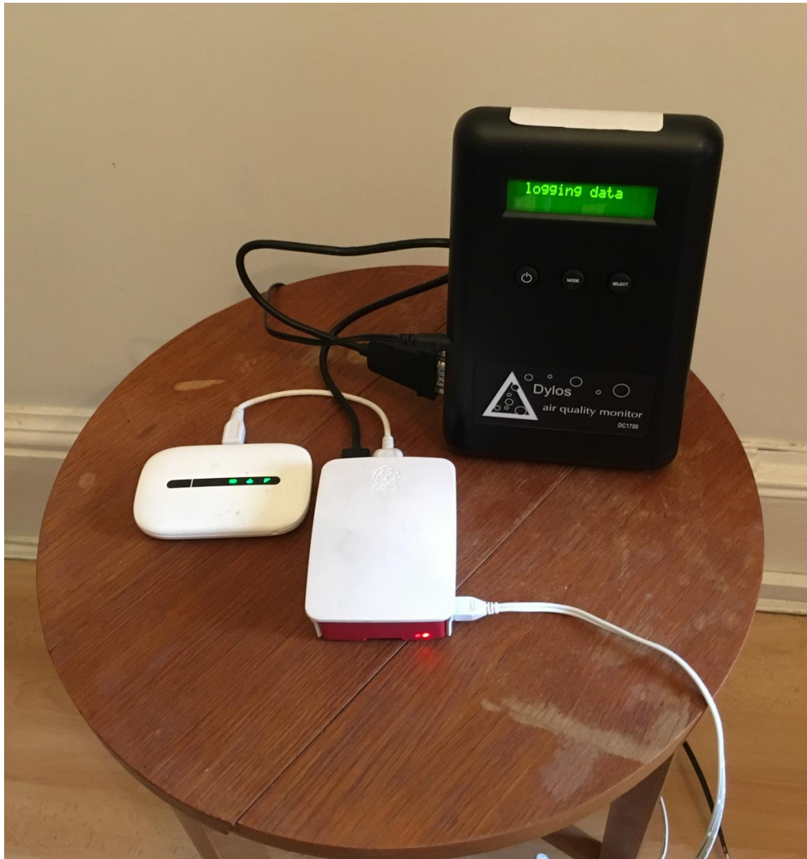
Figure 8 - a RAPID monitor installed and functioning.
