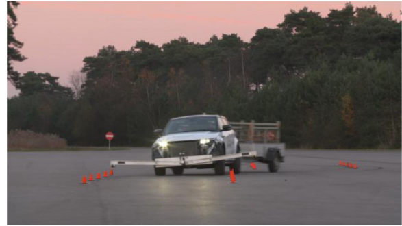
Fig. 9. The vehicle demonstrator with trailer A during an obstacle avoidance test at the Lommel proving ground.
