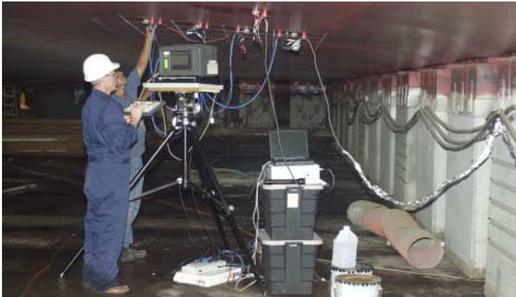
Figure 7 ENM instrumentation positioned under an aircraft carrier bottom for examination of organic coating.
