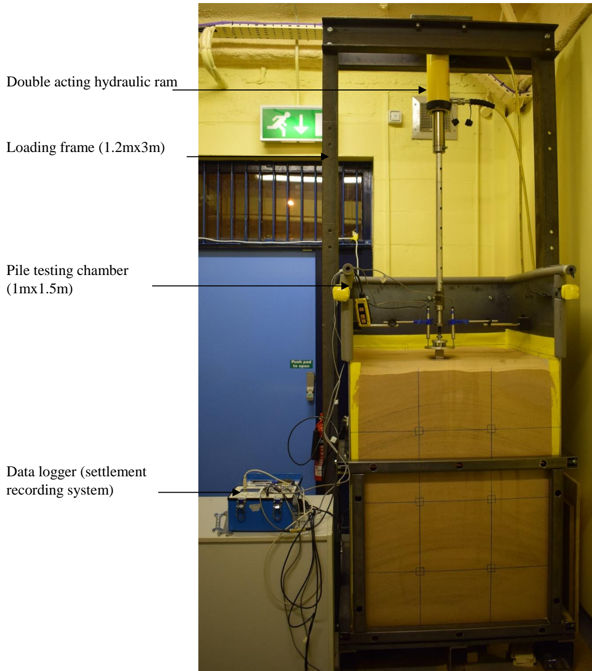
Fig. 3. Schematic view and dimensions of the experimental test setup.
