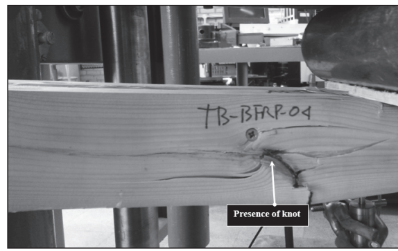
Fig. 8. Observed tensile failure of specimen TB-BFRP-04
