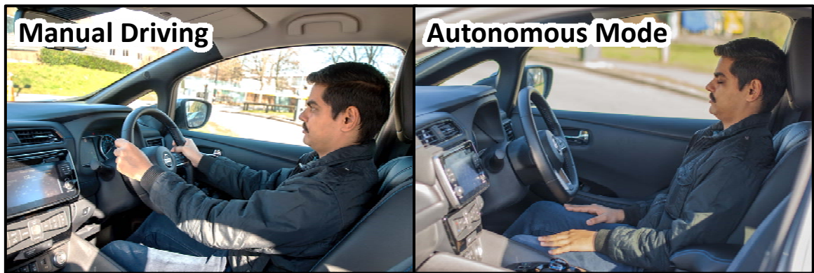
Fig. 1. Manual driving assumes hand, feet and head position in a standard posture. In autonomous mode, these assumptions may no longer hold.
