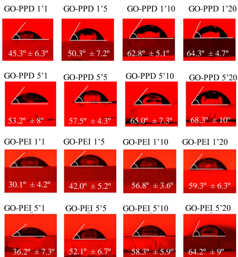
Figure 8. Water contact angles for the crosslinked films.
