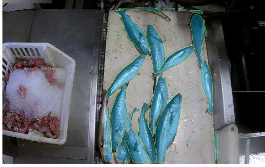
Figure 4: Instance segmentation applied to a frame from footage from Vessel R (research vessel); the blue labels are generated automatically
