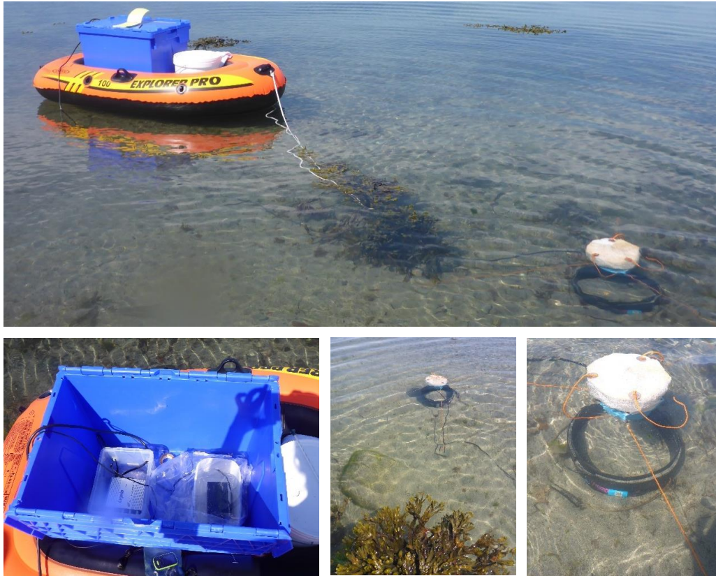
Figure 7-2 Sound set-up. Top: Complete sound set-up on the rubber dinghy. Bottom left: Sound equipment in waterproof boxes and bags. Bottom centre and right: Underwater speaker floating on Styrofoam and held at the same distance to the substrate and sea surface by dive weights (30 cm).
