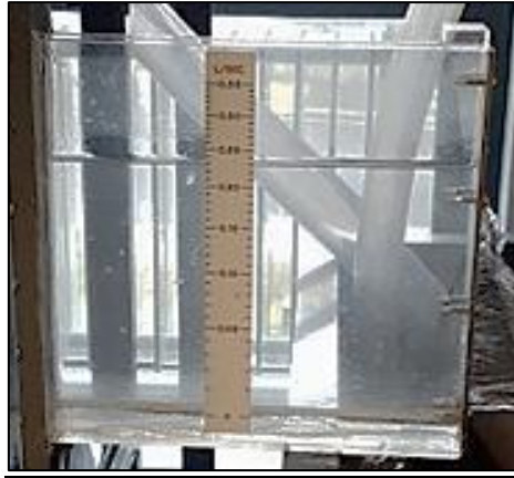
Figure 3: Discharge-measuring device on hydrology bench
