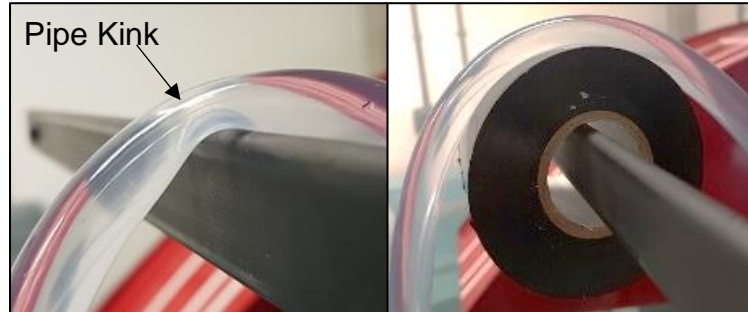
Figure 5: Tape roll to prevent pipe kinking.
