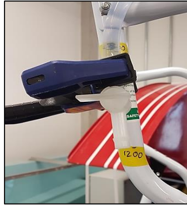
Figure 7: Pipe tap clamped at 1200mm total head
