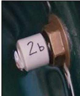
Figure 4: 2mm orifice insert
