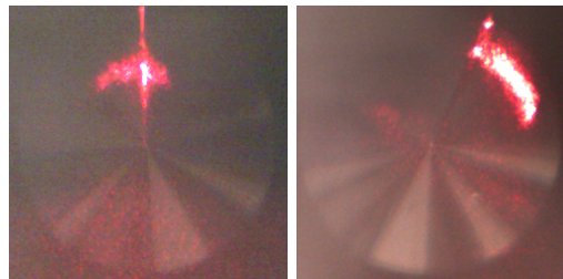
Figure 5: Captured images of the cone mirror when the laser is at 0^\circ and 45^\circ .
