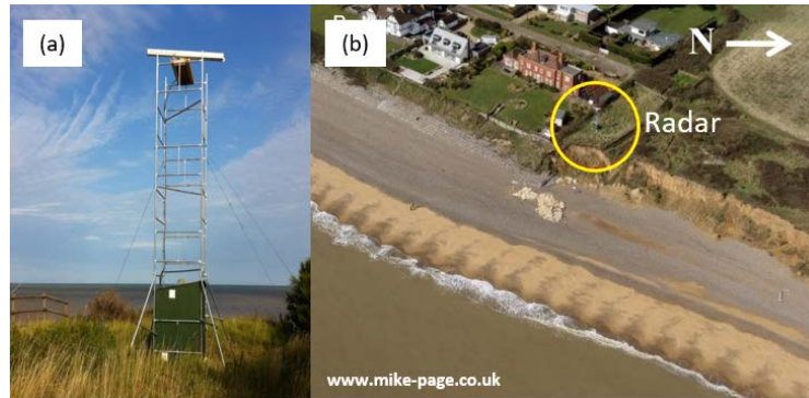
Fig. 3. X-band radar: (a) deployed on 5m tower; and (b) the elevated location on the coast.
