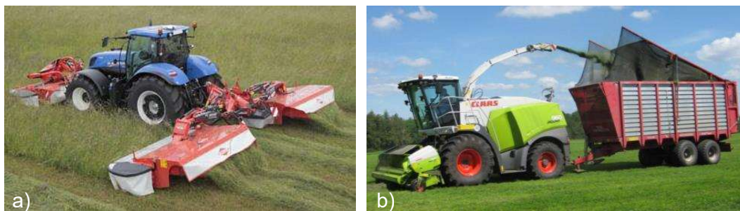
Figure 6. In (a) Triple gang mower of the type envisaged for 9- and 12-m systems. In (b) Example of a self-propelled harvester loading into a towed trailer.
