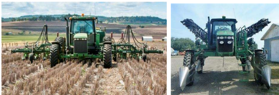
Figure 3. A 8400-series John Deere CTF-compatible tractor (left) with front and rear axles extended to 3-m. Note the tractor positioned on the permanent traffic lanes of a 9-m module CTF system in no-tillage. The machinery width ratio is 3:1, that is, 9-m front combine harvester and planter bar, and 27-m boom width sprayer (right), also with both axles extended to 3-m.
