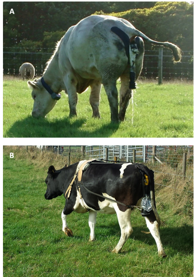
Fig. 1. Attachment of urine sensor to the cow: A, showing initial configuration using Velcro straps glued to cow; B, final configuration using a harness with top and side straps to support sensor weight and minimise lateral movement. GPS collar also shown on the beef cow in A.
