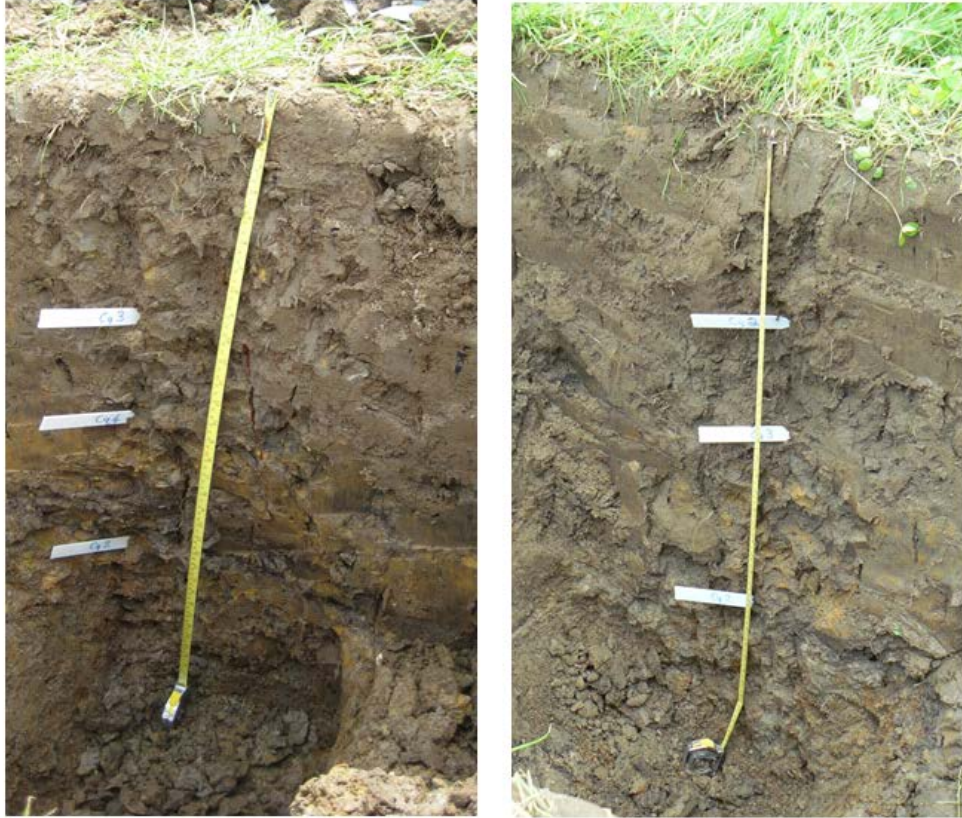
Figure 1. Profiles showing the labels marking the boundaries between layers of differing Sq. The soils are poorly drained eutric gleysol, compacted (left) and not compacted (right), Crichton, Dumfries. They are described in Table 2.
