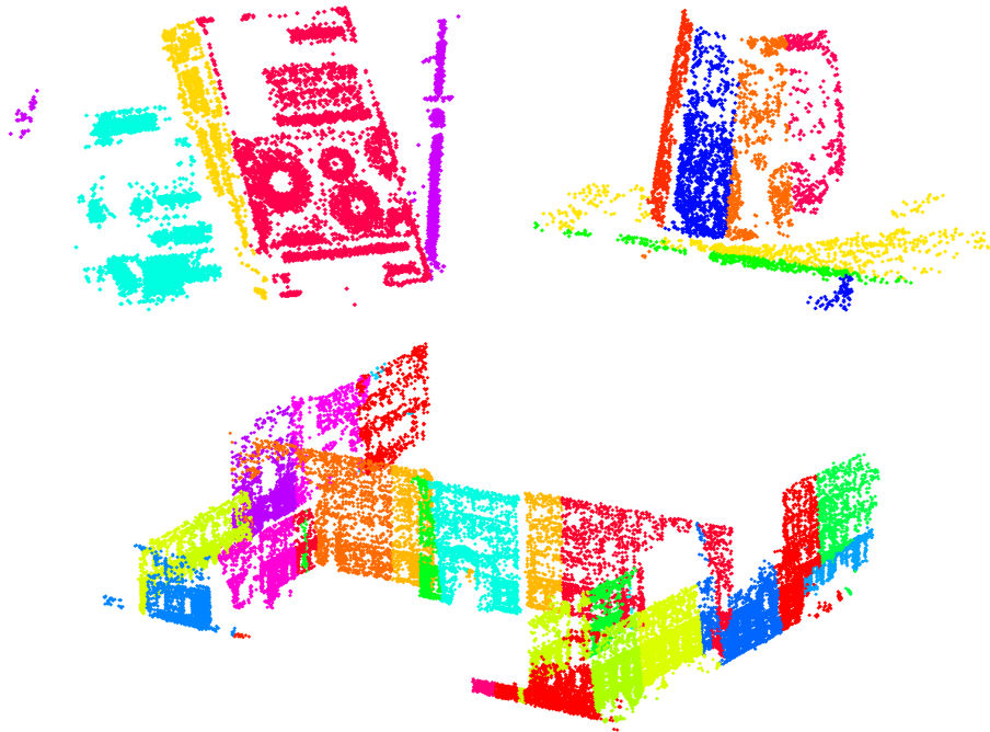
Figure 6: Three segmentation examples on an object-centered scene (top) and a building (bottom). The datasets are the Book , Pot and CAB datasets that can be seen in Figure 10. Each planar patch is in a different color. We can see that the curved surface of the pot is correctly approximated by a set of planar patches.
