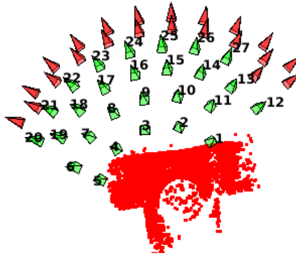
Figure 17: Test with the Pot sequence: cameras in red are used to build the SfM model, whereas cameras in green are used as tests for pose computation.
