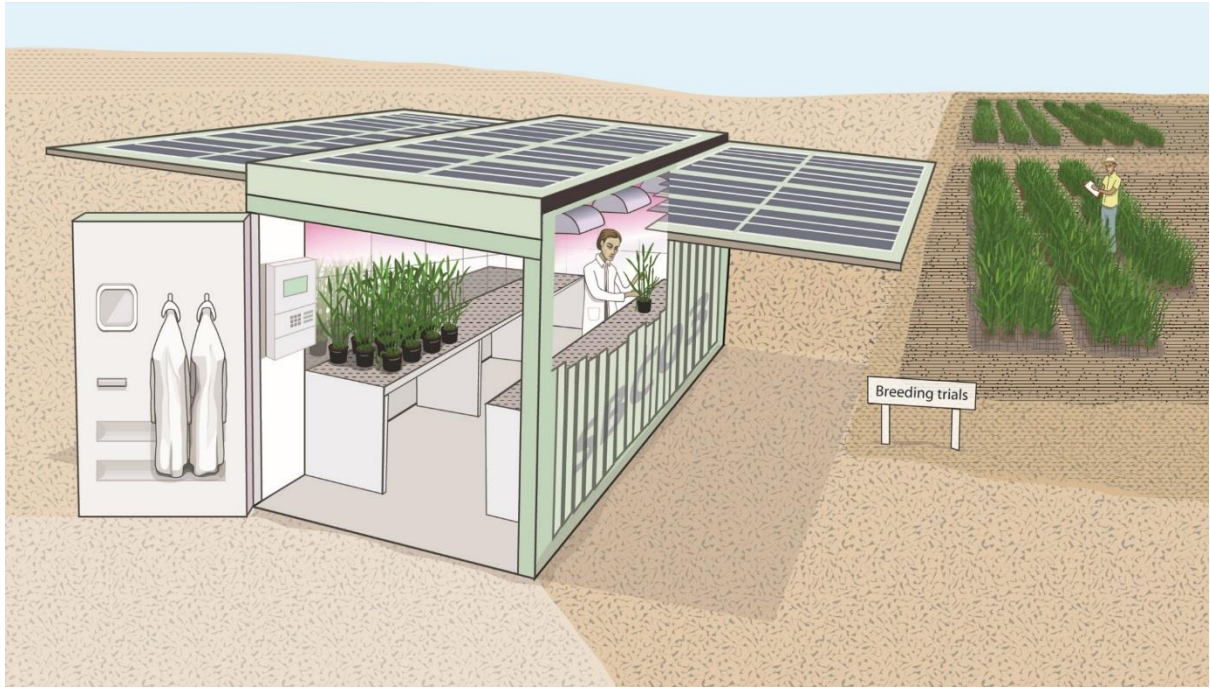
Fig. 3 Artist's impression of a speed breeding capsule made from a disused refrigerated shipping container and deployed for accelerated orphan crop breeding.
